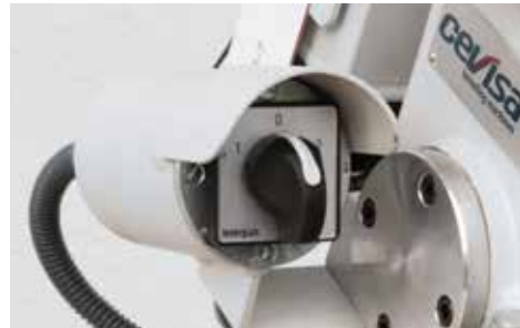
Interruptor inversor. Reverse-switch.
